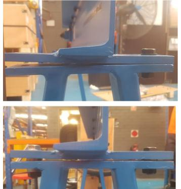
It is also recommended to have the hand shears bolted down. Ensure the shears are levelled correctly before bolting down, otherwise this will cause a twist in the bottom blade, and poor cutting performance.
